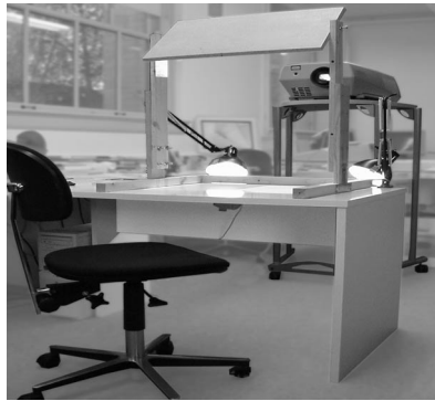
Figure 1. One of our Gesture Modelling configurations: camera and gesture space beneath the desk, with lights, projector and mirror displaying the model image on the desk top.
