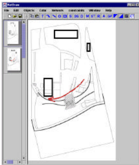
Figure 2. The NetDraw graphics screen with a scanned image underlay, geometric objects, and an ephemeral gesture (red arrow). Two snapshots from the design history are on the left; the command menu bar is on top.
